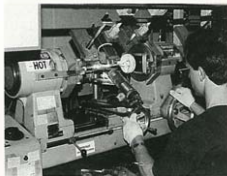
Renaat Beelen shows the careful control of the lathe which is required to ensure the correct formation of the lamp bulb.
