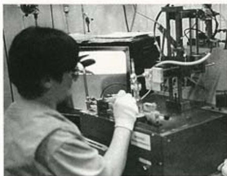
Hilde Kinnaer demonstrates the fine work of correctly placing the electrodes in the bulbs of a 1200W single-ended lamp before the seal is made, automatically.
