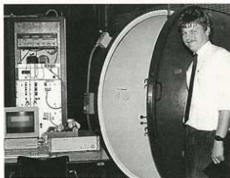
Patric Geubbelmans alongside an Ulbricht sphere dedicated to the test procedure for the photometric and electric performance of each lamp.
